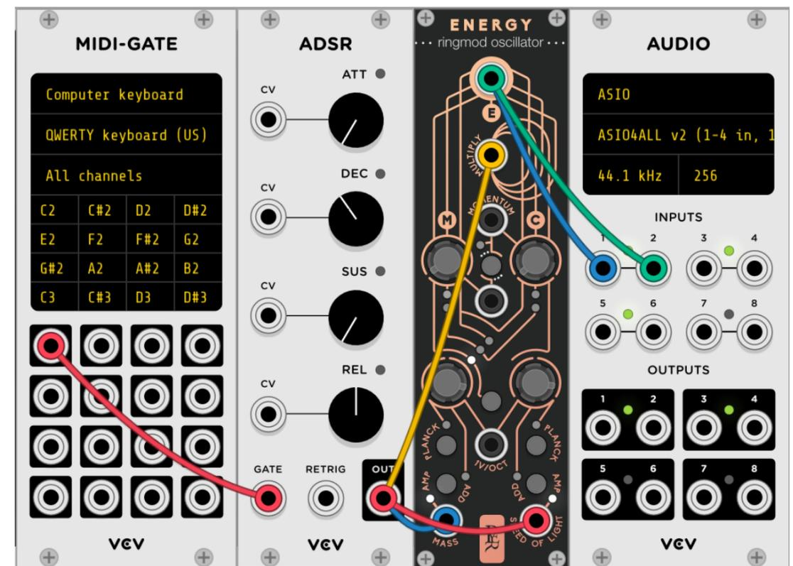
**Percussion:** in amp mode, fall from the knob position to the centre point, for a decay from aggressive to soft tone.
