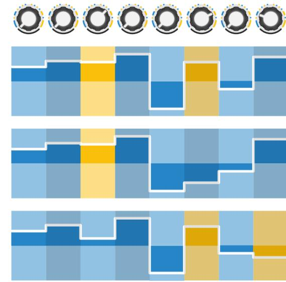
The probabilities for each step can be controlled all together by the **knob on the top**, which will add an offset to each knob. This knob is CV controllable with a  $-5V$  to  $+5V$  range.
