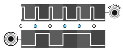
It has two uncorrelated internal random generators, one for each **CV output**. They can be added to the original signal or used on their own.
