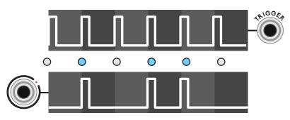
• Hold trigger: the gate is open when random is active.
